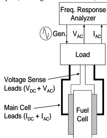
**Figure 1. Instrumentation for EIS of fuel cells.**
