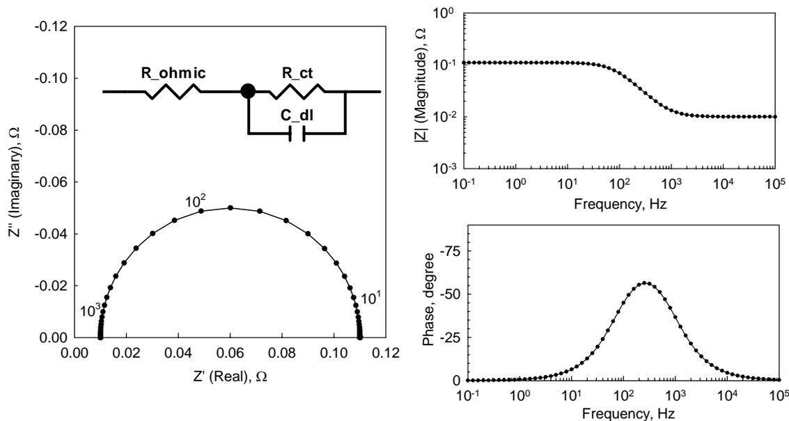
**Figure 2. Impedance plots for the indicated simple RC circuit where  $R_{ohmic} = 0.01 \Omega$ ,  $R_{ct} = 0.1 \Omega$  and  $C_{dl} = 0.02 F$ . For clarification, 3 frequencies ( $10^3$ ,  $10^2$  and  $10^1$  Hz) are labeled in the complex plane (Nyquist) plot.**
