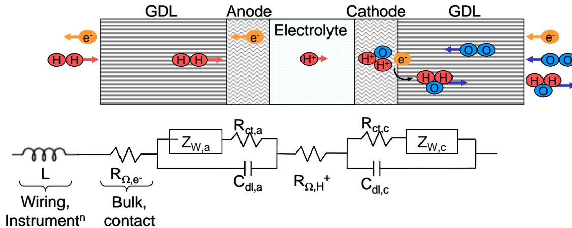
Key: GDL = gas diffusion layer, dl = double layer, ct = charge transfer, a = anode, c = cathode.
