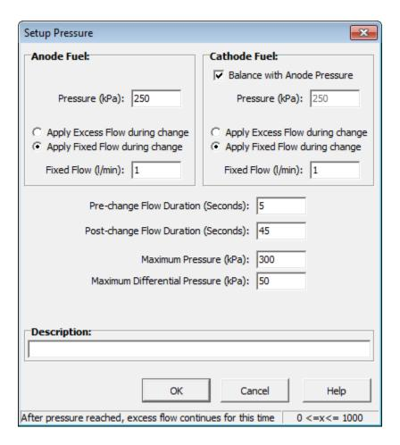
The **Anode** and **Cathode Pressure** set-points can be entered separately.
