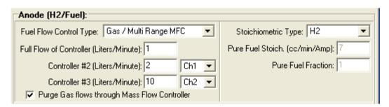
**Controller #2 (Liters/Minute)** sets the full flow size of the second main gas controller. The second controller must be larger than the primary controller. The **Channel Number** selects the Reformate simulator channel that will be used to control the second main gas controller.
